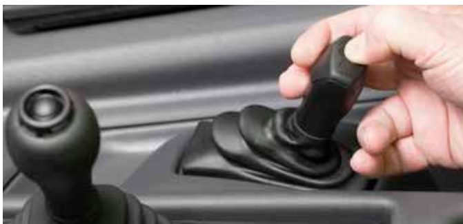
Body hoist lever with boost button
