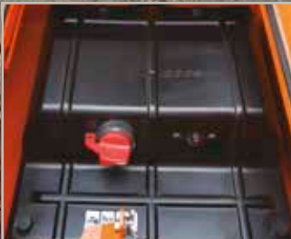
Battery cut-off switch
