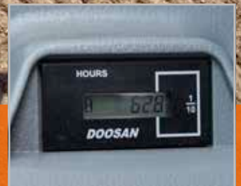
Hour meter (from ground level)
